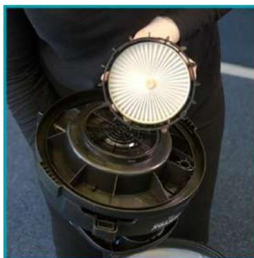
After every use check the dust bag and if full replace. Check the filter bag and filter to ensure there are no blockages.
