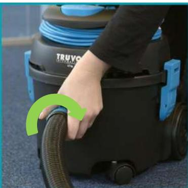
Attach the vacuum hose by turning in a clockwise direction.
