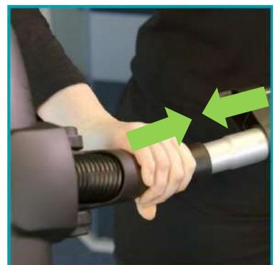
Attach the floor tool to the wand.
