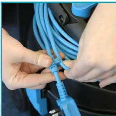
Always unplug the machine after use. Check the power cable for any wear or damage and wrap the cable around the machine.
