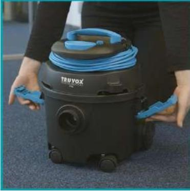
Pull the two latches on either side of the machine.
