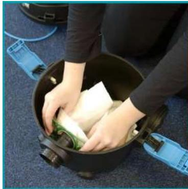
Install a new bag by securely fitting onto the nozzle.
