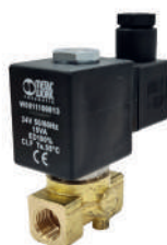
ELECTROVÁLVULA 2/2 ACL 1/4" 24 V 50/60 Hz N/C
